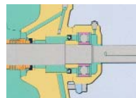
7b: Inboard component mechanical seal
